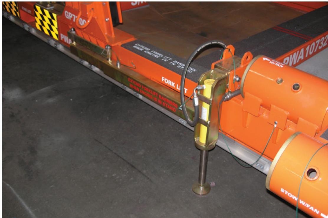
Figure 5.2-4 Jacking Leg - Extended (for leveling and caster deployment/stow)
