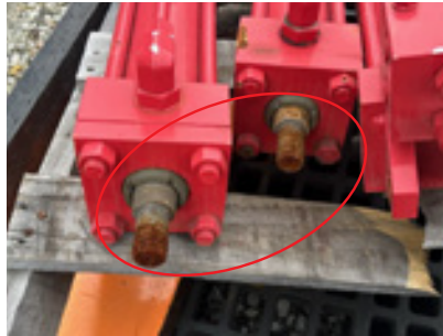
Hydraulic Cylinder Damage
