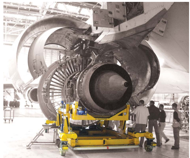
Uplift Shipping Stand Interfacing with Bootstrap System Engine OEM P/N: 9C6025 AGSE P/N: AGSE-E102
