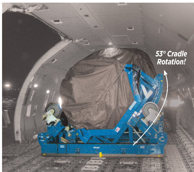
Roll-Over Shipping Stand in Low Profile Position loaded onto the Main Deck of a Boeing 777 Aircraft
