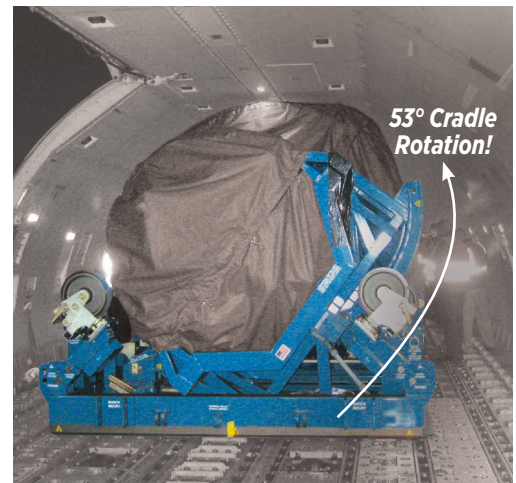
GEnx-1B Roll-Over Shipping Stand on a Boeing 777 Aircraft Engine OEM P/N: 11C3359 AGSE P/N: AGSE-E184
