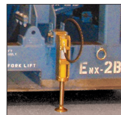
Jacking Leg Deployed
