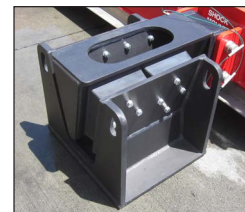
External Shock-Absorbing Mount
