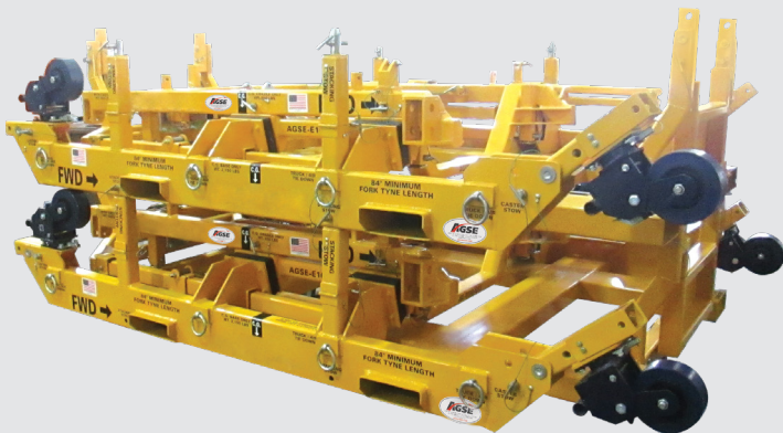
Empty Shipping Stands in Stacked Configuration AGSE P/Ns: AGSE-E094/-E169
